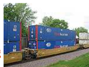
Expand Image Allowing trains to carry double-stacked containers will mean more cargo is moved and fuel is saved.
